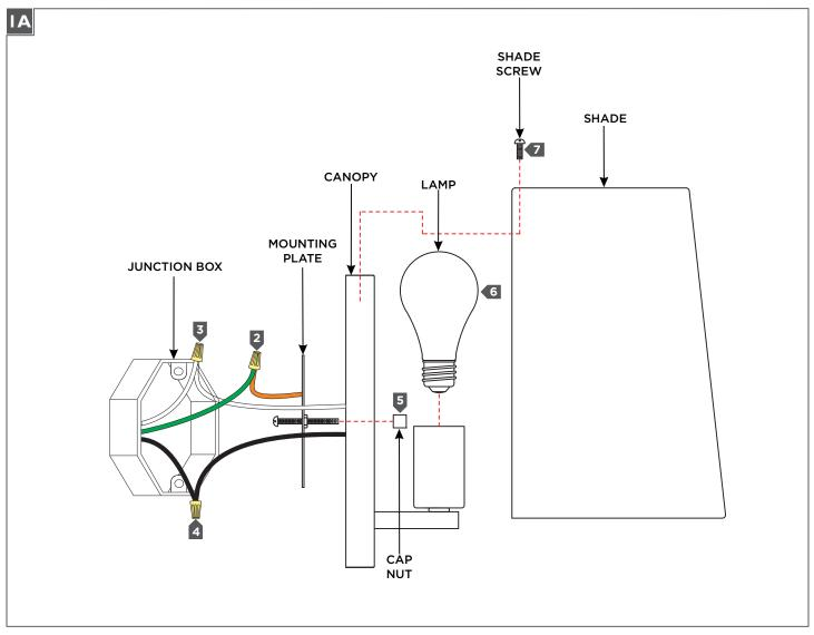
**1** Secure the mounting plate to the junction box.
